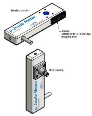
The adapter plate allows screwing a stand underneath the  $\mu$ -Joule Meter in order to achieve more stability during the measurement process; the plate contains two mounting holes, for metric or inch screws.
